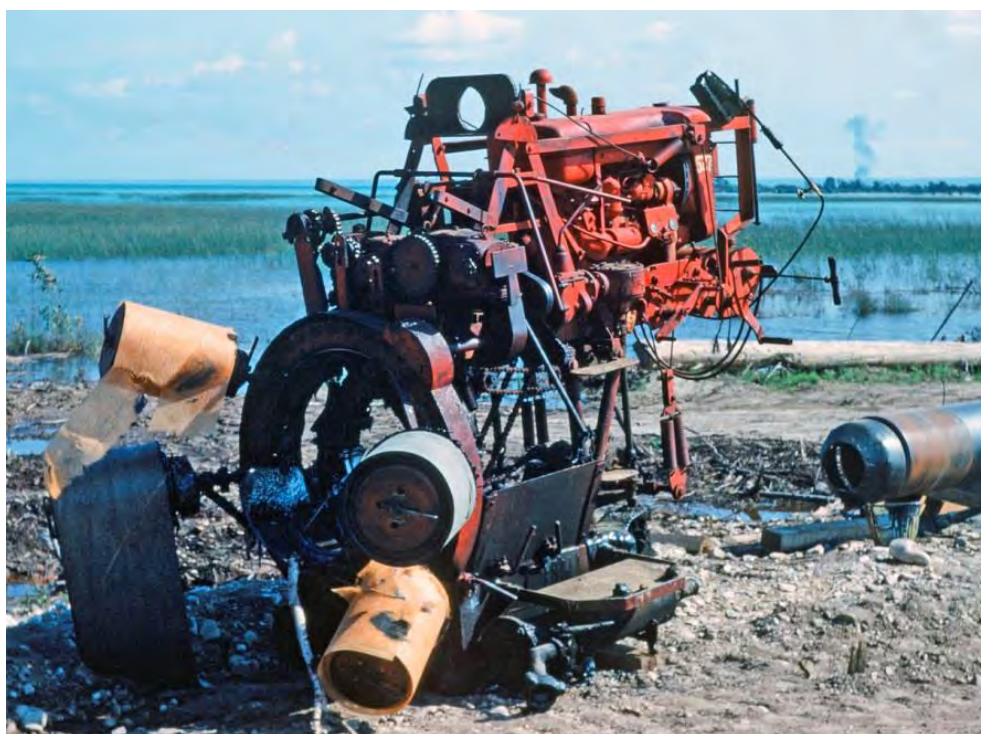
Figure 2. Trudgen Photo of Pipe Wrapping Machine (00010370012.tif)
