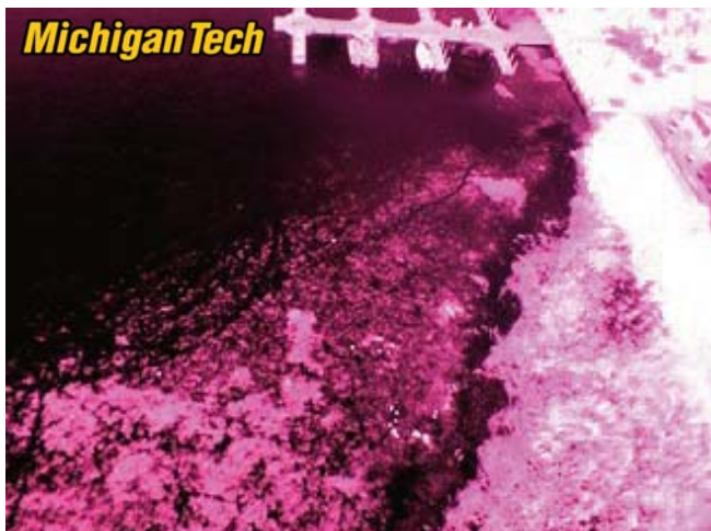
Michigan Tech Les Cheneaux study by Michigan Technological University measures light reflectance to identify invasive weed species.
